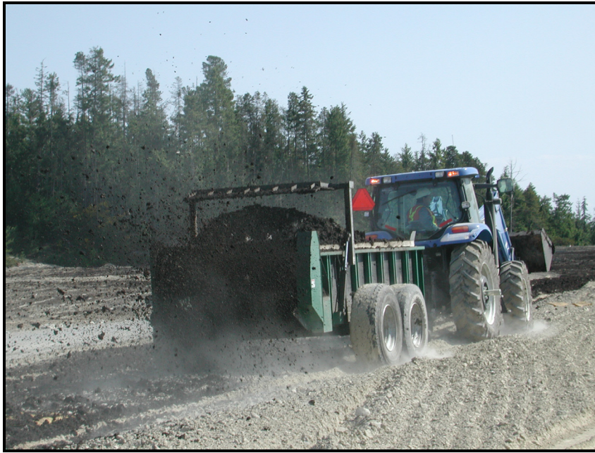
Photograph 1: Biosolids can be uniformly applied using conventional farm equipment, such as the tractor and rear-discharge manure spreader pictured here.
