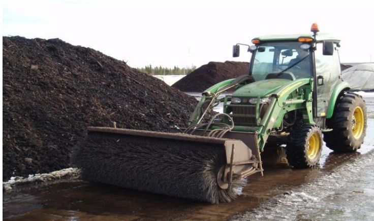
Figure 3. Cleaning with tractor-mounted broom.
