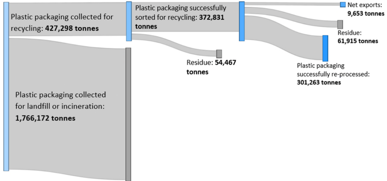
Figure 2: Flow of plastic packaging through the recycling stream, 2018
