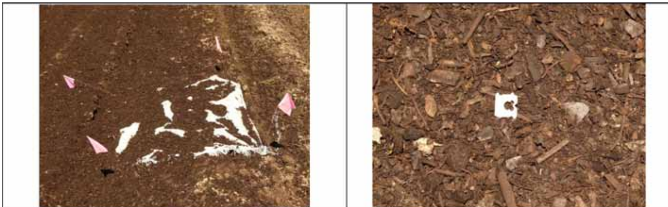
An example of calibration – double the speed does not result in double the rate.
